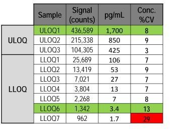
The LOB was determined by running 20 replicates of zero calibrator per plate and calculating the concentration corresponding to the average zero calibrator signal plus 2.5 standard deviations. The LLOQ and ULOQ were determined by running six plates on two days with four replicates per plate. LLOQ was defined as the lowest concentration with a total CV of 20% or less. ULOQ was defined as the highest concentration with a total CV of 20% or less.
