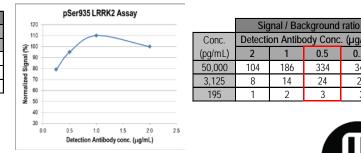
The graphs show representative data obtained from the analysis of three calibrator levels (STD2, STD4, and STD6) as a function of detection antibody concentration. The signal at each calibrator level is normalized to the signal at the highest detection antibody concentration (2  $\mu$ g/mL). The tables to the right of the graphs report the signal to background ratios, which were the deciding factors for selecting the optimal detection antibody concentration.
