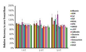
Controls at different levels were made by spiking calibrator into urine. These controls were tested for 5 freeze/thaw cycles. Data showed some controls were not stable at 5 freeze/thaw cycles. Based on these data, MSD does not recommend multiple freeze/thaw cycles for controls.
