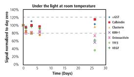
Detection antibodies were stored with or without light exposure at room temperature up to 26 days. Data from KIP3 showed some detection antibodies are sensitive to light, but all have good long term stability in the dark. MSD recommends storing detection antibody in the dark at 4°C.
