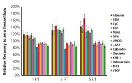
KIP3 and KIP5 calibrators were tested for 5 freeze/thaw cycles. Data showed some analytes, including albumin, B2M, cystatin C and NGAL, are not stable for multiple freeze/thaw cycles. MSD does not recommend multiple freeze/thaw cycles for calibrators.
