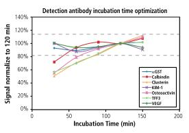
A protocol time tolerance study was conducted with a series of time points. 2 hours incubation time for calibrator or detection antibody was optimal. The data demonstrated that assay incubation time can vary by 30 min in either direction with signals remaining within 15%.
