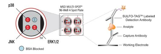
**Figure 1.** Spot diagram showing placement of analyte capture antibody. The numbering convention for the different spots is maintained in the software visualization tools, on the plate packaging, and in the data files. A unique bar code label on each plate allows complete traceability back to MSD manufacturing records.
