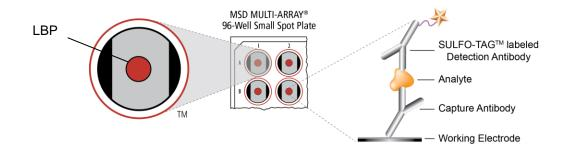
*Figure 1.* Sandwich immunoassay on MSD platform. A unique bar code label on each plate allows complete traceability back to MSD manufacturing records.
