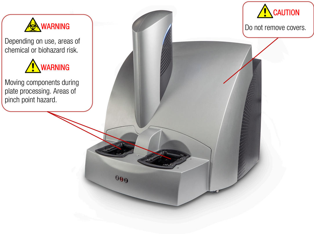
Figure 3.1 MESO SECTOR S 600MM Hazards
