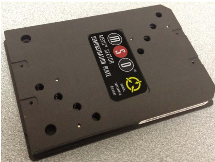
For the SECTOR S 600, sectors 3 and 4 (Figure 3:11) of the demonstration plate have LEDs that test the CCD camera in the instrument. The remaining four sectors of the plate contain known electronic components for testing the electrical functioning of the instrument across its range of operation. The demonstration plate can be used without any chemical reagents, either to check instrument function at the start of each day or as a tool for demonstrating the instrument and software to new users.
