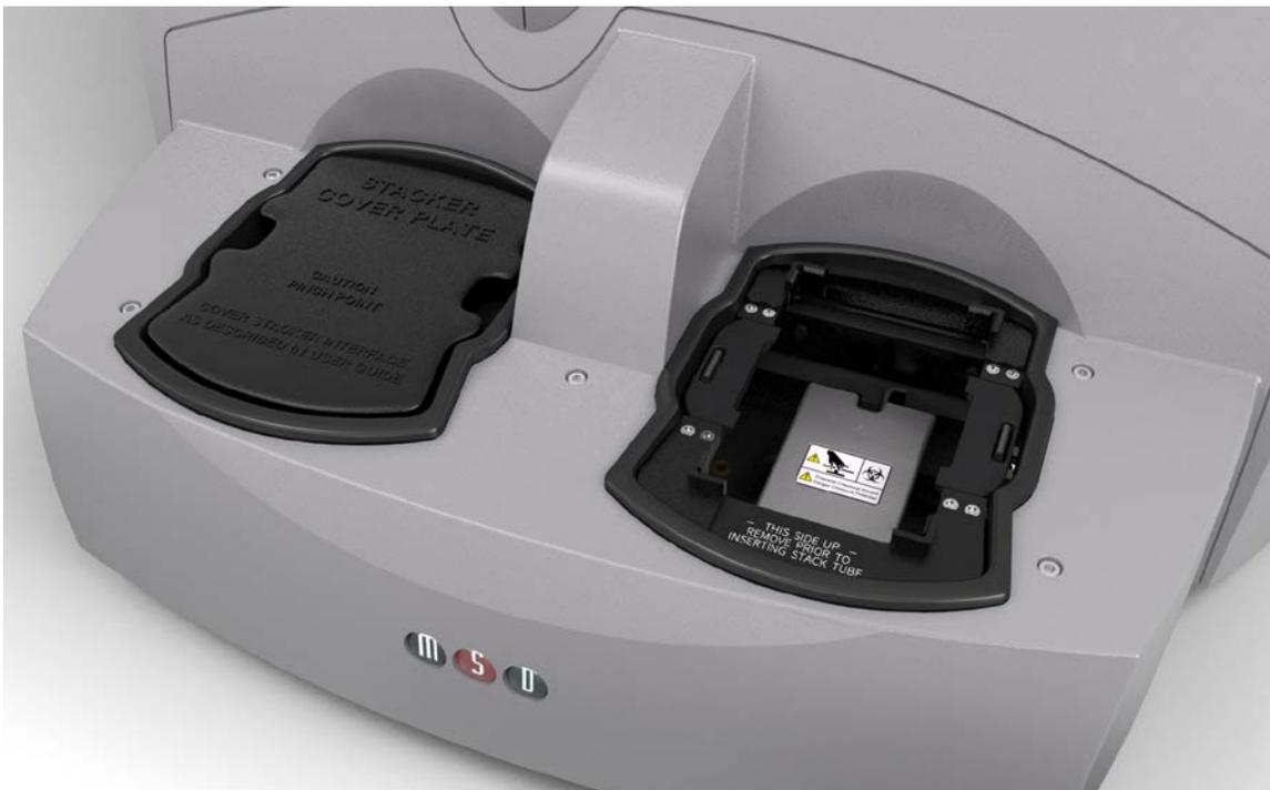
6. Place the demonstration plate in the single plate adapter with the chamfered corners of the plate facing into the instrument (Figure 5:7).
