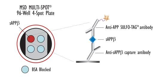
Recombinant human sAPP $\beta$  was purified from mammalian cells (>95% pure) and diluted in denaturing assay diluent. Samples were added to MSD MULTI-SPOT 4 spot plates coated with anti-sAPP $\beta$  antibody on one of four spatially distinct electrodes per well. sAPP $\beta$  protein was detected with anti-APP antibody (22C11), labeled with MSD SULFO-TAG reagent.
